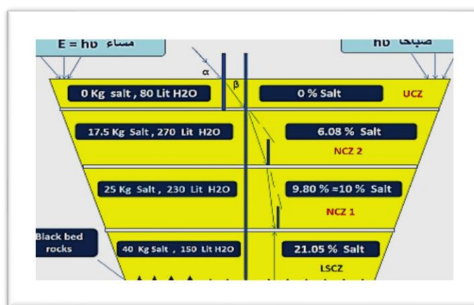
Fig.1. shows the studied solar pond layers and their content of water and salt
